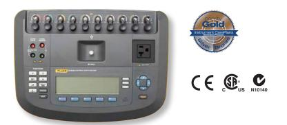
The multifaceted ESA620 Electrical Safety Analyzer performs all primary safety tests including mains voltage, protective earth resistance, insulation resistance, device current, earth, chassis, and patient leakages as well as several additional leakage tests to comply with standards of choice.
